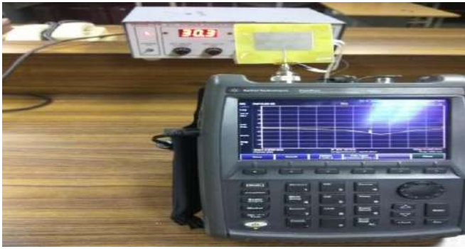
Fig 3(a) Experimental setup to measure the return loss of rectangular microstrip antenna with teflon material
